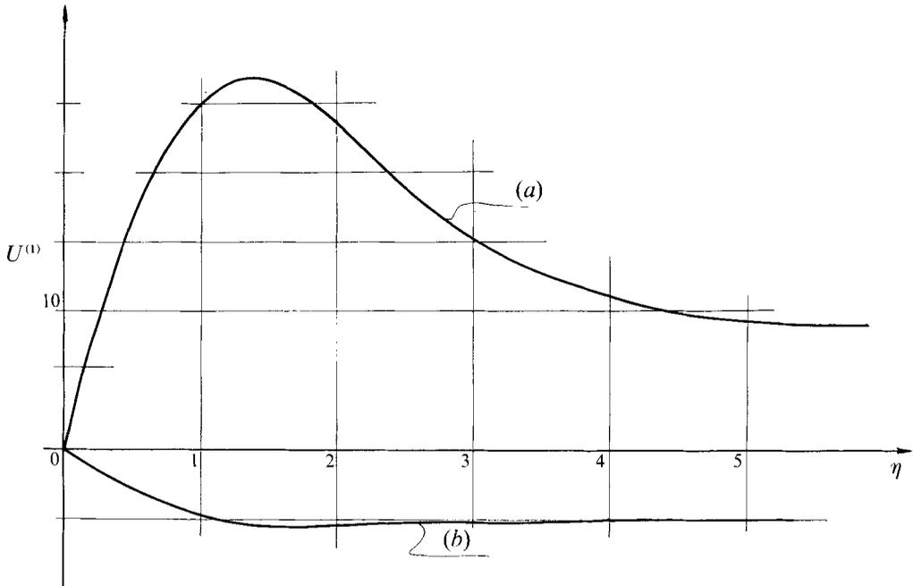
FIGURE 3. Second-order correction for the streamwise velocity in the boundary layer for  $x = 2.5$ : (a) subcritical flow ( $F = 0.75$ ); (b) supercritical flow ( $F = 1.5$ ).
