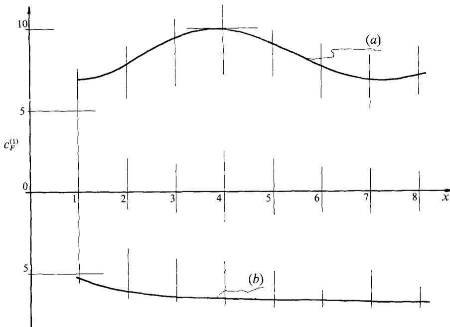
FIGURE 10. Second-order correction for the coefficient of integrated skin friction: (a) subcritical flow ( $F = 0.75$ ); (b) supercritical flow ( $F = 1.5$ ).
