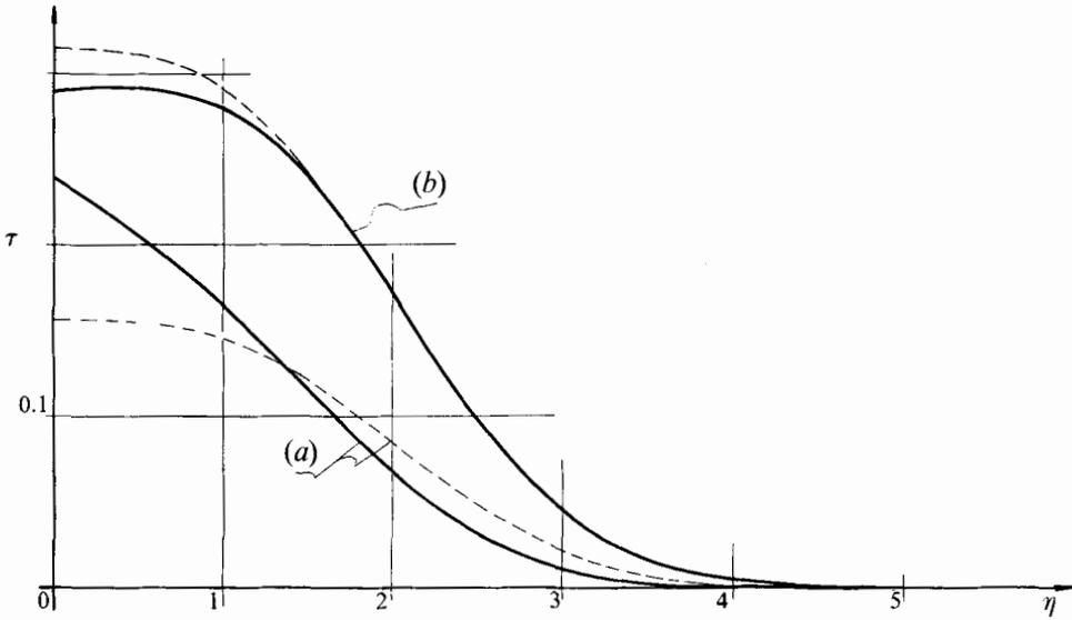
FIGURE 6. Total shear stress in the boundary layer for  $x = 2.5$ ,  $1/R^{\frac{1}{2}} = 0.006$ : (a) subcritical flow ( $F = 0.75$ ), (b) supercritical flow ( $F = 1.5$ ); with the second-order correction (—), without the correction (-----).
