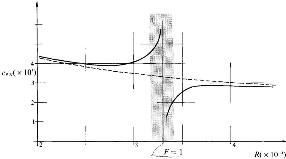
FIGURE 12. Coefficient of integrated skin friction as a function of Reynolds number (for water,  $x = 5$ ,  $h = 0.05$  m): with the second-order correction (—), without the correction (-----).
