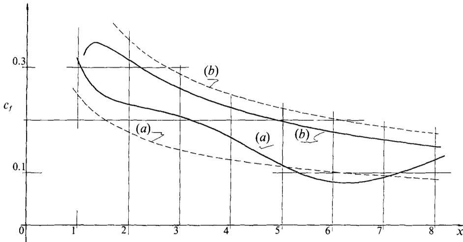
FIGURE 8. Coefficient of local skin friction for  $1/R^{1/2} = 0.0035$ : (a) subcritical flow ( $F = 0.75$ ), (b) supercritical flow ( $F = 1.5$ ); with the second-order correction (—), without the correction (-----).
